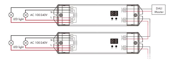
If output connect with capacitive or inductive load, the maximum output current only up to 5A. If output connect with resistive load, the maximum output current may up to 8A.
