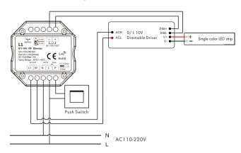
Connect with 0/1-10V dimming driver (use AC OUT and relay or contactor)
