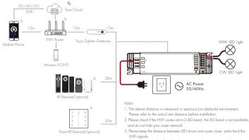
Continuously switch off and on the power supply two times rapidly, It will change 3 levels color temperature (WW, NW and CW) in sequence.
