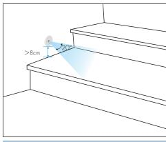
When installing on stairs, install at a height of 8cm or more, as far away from the foot elevation as possible.
