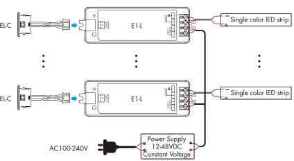
For multiple applications, it is recommended to set the delay time of all laser sensor head to 5 or 10s. Realize the sequential switching control of multiple lights according to the direction of human walking.
