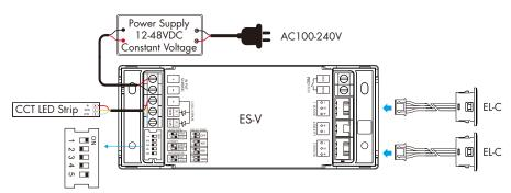
The ES-V constant voltage controller is connected to two laser sensor head which are installed on each side of the corridor.
