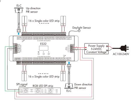
Connect the ES32 sensor stair light controller to two laser sensor head, which are installed at the top and bottom of the stairs. Set the delay time of the laser sensor head to 2s (default).
