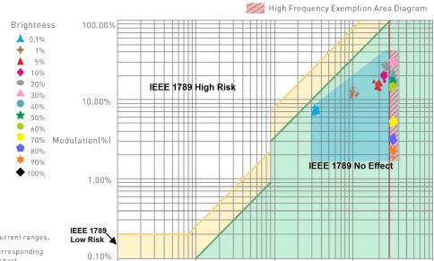
$\label{thm:marks} \mbox{Marks in the right chart were tested results of different current ranges.}$
